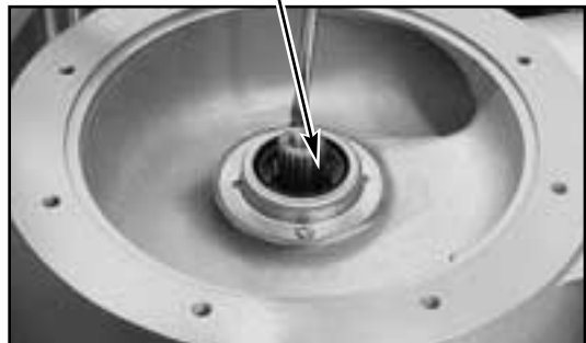
Seal and Motor Housing locations plus Permatex Sealing area. "1" and "2" Critical Sealing areas shown.
