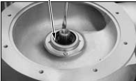
Seal and Motor Housing locations plus Permatex Sealing area. "1" and "2" Critical Sealing areas shown.
